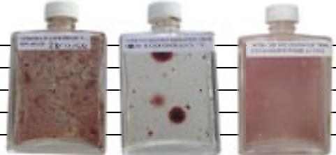
■ Fuel Doctor is said to work by absorbing water and dispersing microbes, enabling them to pass harmlessly through filters. Fuel Doctor performed reasonably well in the decontamination trial, albeit with the highest dose rate (0.5%) of any product. It gave a 50-fold reduction after three hours and a further 150-fold reduction after three days. Filterability improved to a ratio of 1.65.
