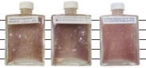
■ Fuel Set claims to prevent diesel bug by absorbing water in the fuel, however the manufacturers suggest several successive treatments or on-going application may be required, so the results of a three-day once-only application would be insubstantial. In the decontamination trial Fuel Set gave no significant reduction in microbial count and the flow ratio was 3.2. In the prevention trial the product did nothing to prevent microbial growth.
