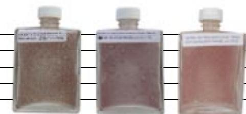
■ Soltron claims to kill microbes by using enzymes to break them up, allowing the dead matter to pass harmlessly through the filter. We were advised to apply twice the dose recommended in the product instructions, but despite doing this there was no significant reduction in microbes after three days. At a flow ratio of 2.44 filterability was slightly better than the control (2.57).
